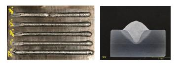
Figure 4. TW-GMAW CTWD sensitivity tests: weld visual appearance (left), and metallographic cross-section of the weld made with ¾-in. CTWD (right).
