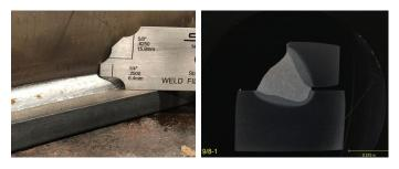
Figure 5. TW-GMAW weld made at a total wire feed input rate of 940 ipm with a travel speed of 25 ipm: weld visual appearance (left) and metallographic cross-section (right).
