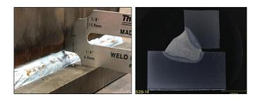
Figure 6. TW-GMAW weld made at a total wire input rate of 1200-ipm WFS with a travel speed of 30-ipm: weld visual appearance (left) and metallographic cross-section (right)
