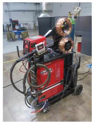
Fig. 1.1 – Welding generator and equipment for HyperFill<sup>™</sup> technology
