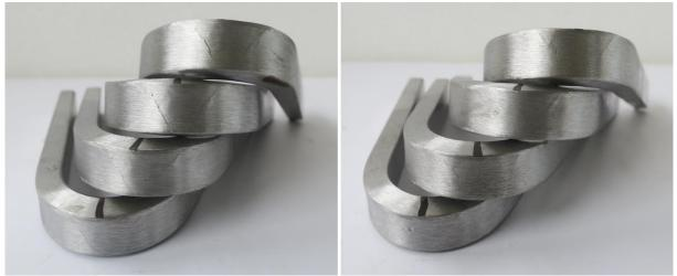
Fig. 3.28 – Specimens submitted to lateral bend test: GMAW on the left, HyperFill™ on the right
