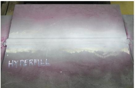
Fig. 3.2.1 – Liquid penetrant inspection on HyperFill<sup>TM</sup> butt joint
