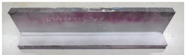
Fig. 3.1.1 – PT on fillet weld realized with HyperFill™
