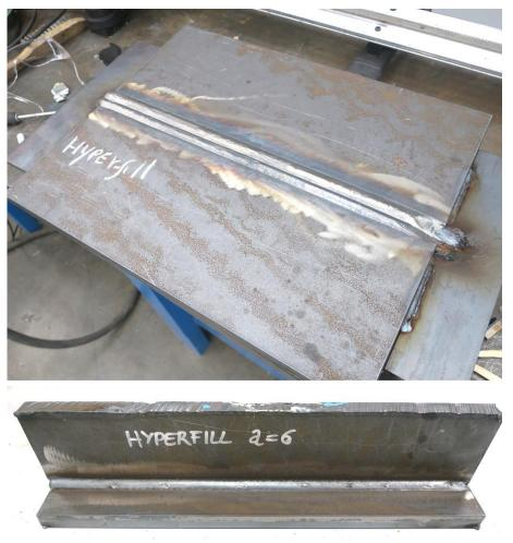
Fig. 2.2.4 – Joints realized with HyperFill<sup>™</sup> process
