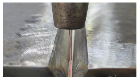
Fig. 2.2.3 – Detail of the twin-wire in HyperFill<sup>™</sup> process
